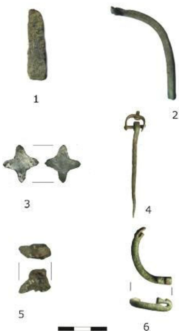
Fig. 5. Waste and intermediate products of non-ferrous metalworking found over 1981–2010 (photo K. Żołędziowski): 1. inv. 189/05P; 2. inv. 3/82P; 3. inv. 637/10P; 4. inv. 382/06; 5. inv. 547/10P; 6. inv. 752/05P
