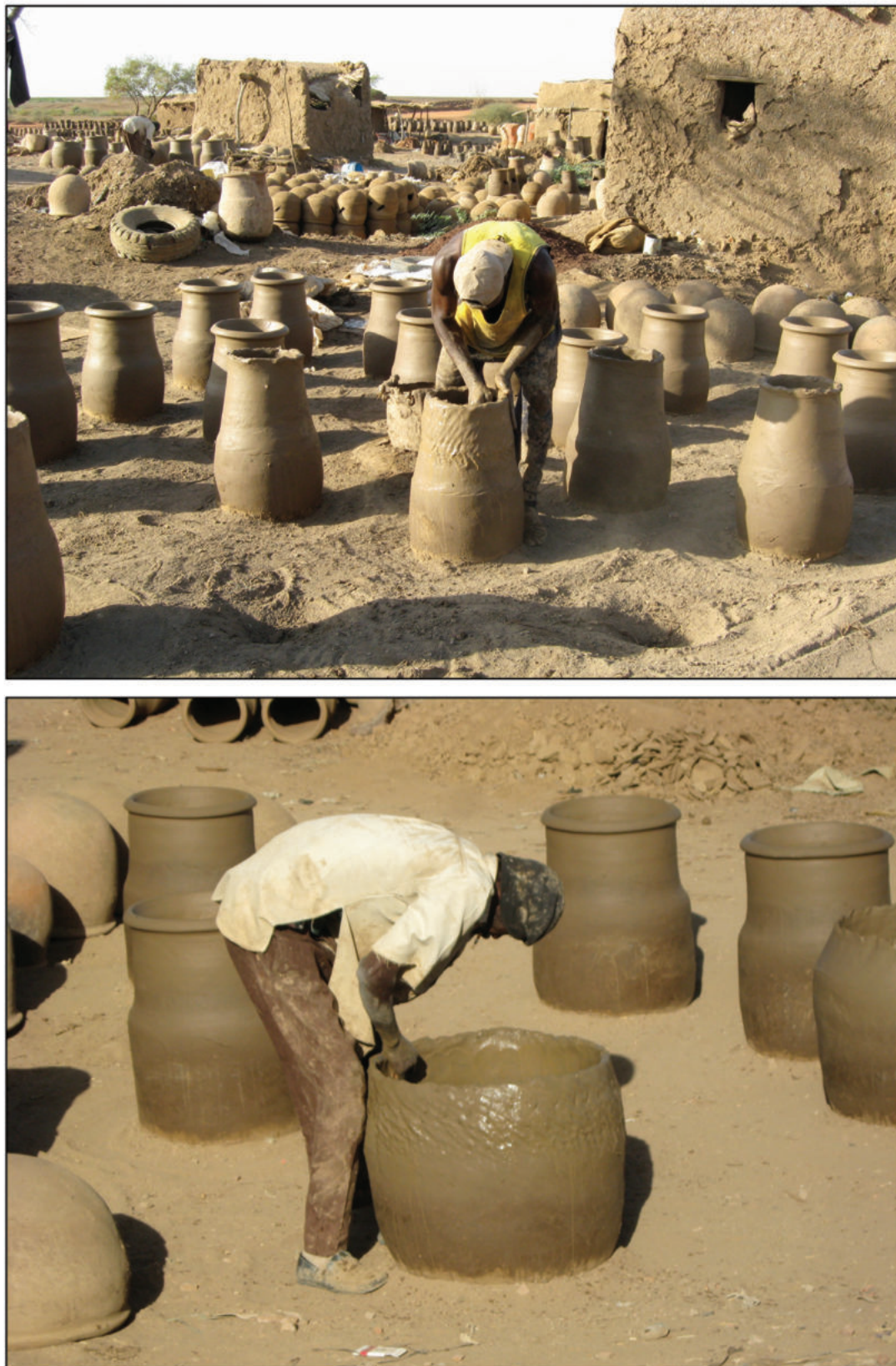
Fig. 4. Orbiting. Potters move around a fixed vessel during both the forming and shaping process. Two pottery workshops at a pottery centre in Wad Medani. Sudan 2008 (photos M. Daszkiewicz)
