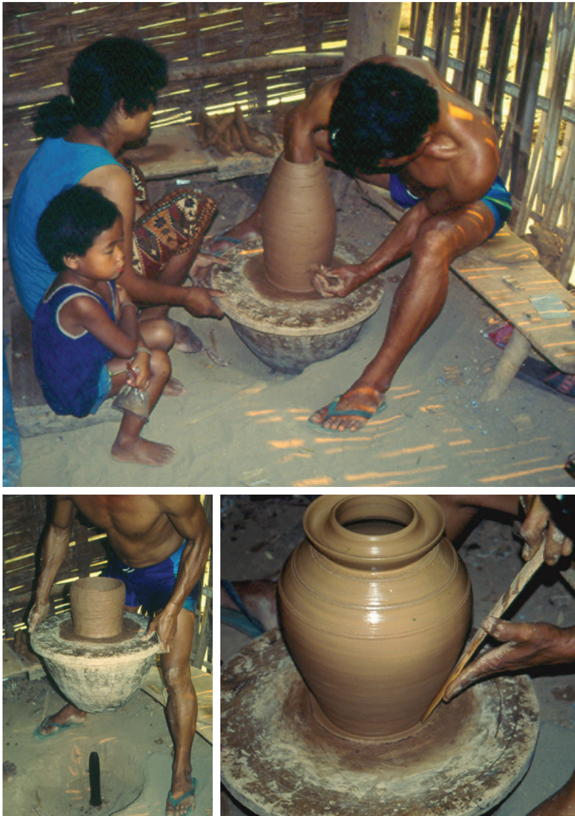
Fig. 6. Wheel-shaped. Coiling: the vessel is built of coils, which are bonded by applying discontinuous pressure, without the help of rotative kinetic energy; thinning and shaping is done with the help of rotative kinetic energy. Hand-operated turntable. Laos 1994 (photos G. Schneider)
