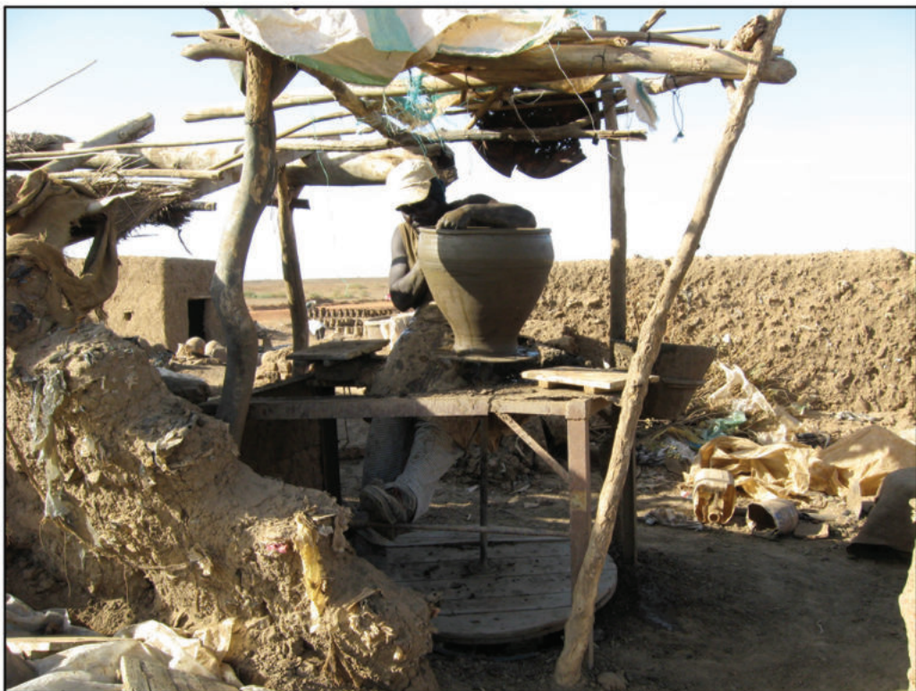
Fig. 7. Wheel-shaped. Coiling: coils are laid and bonded on the wheel and the vessel walls are thinned with the help of rotative kinetic energy, after which the wheel is stopped and the next coil is added. Wad Medani, Sudan 2008 (photo M. Daszkiewicz)
