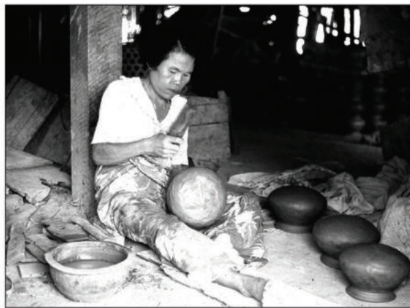
Fig. 3. Handmade. Shaping using the paddle and anvil technique, Laos 1994 (photo G. Schneider)
