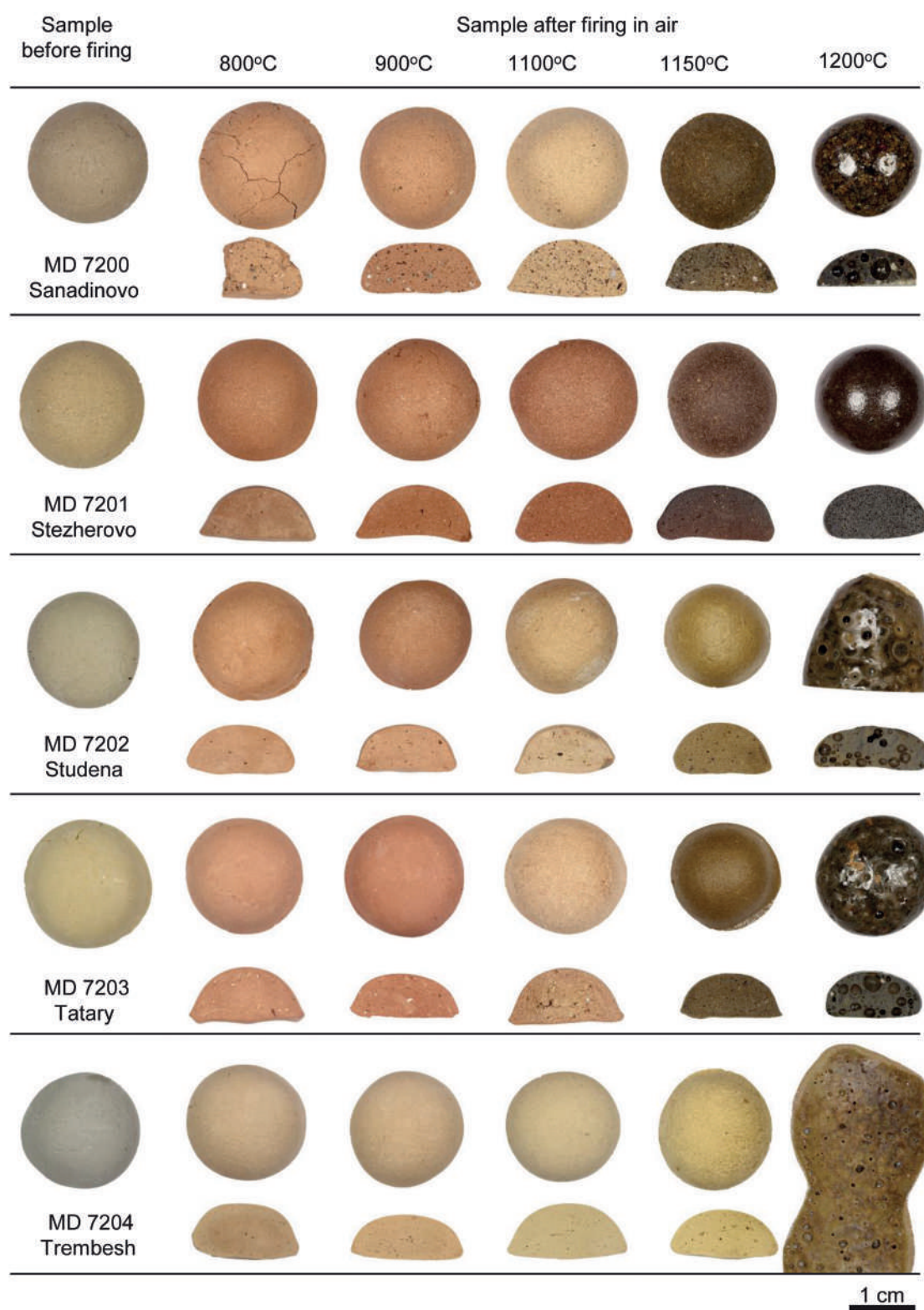
Pl. 13. Firing test, clay samples MD7200–MD7204 (compiled by H. Baranowska and M. Daszkiewicz)
