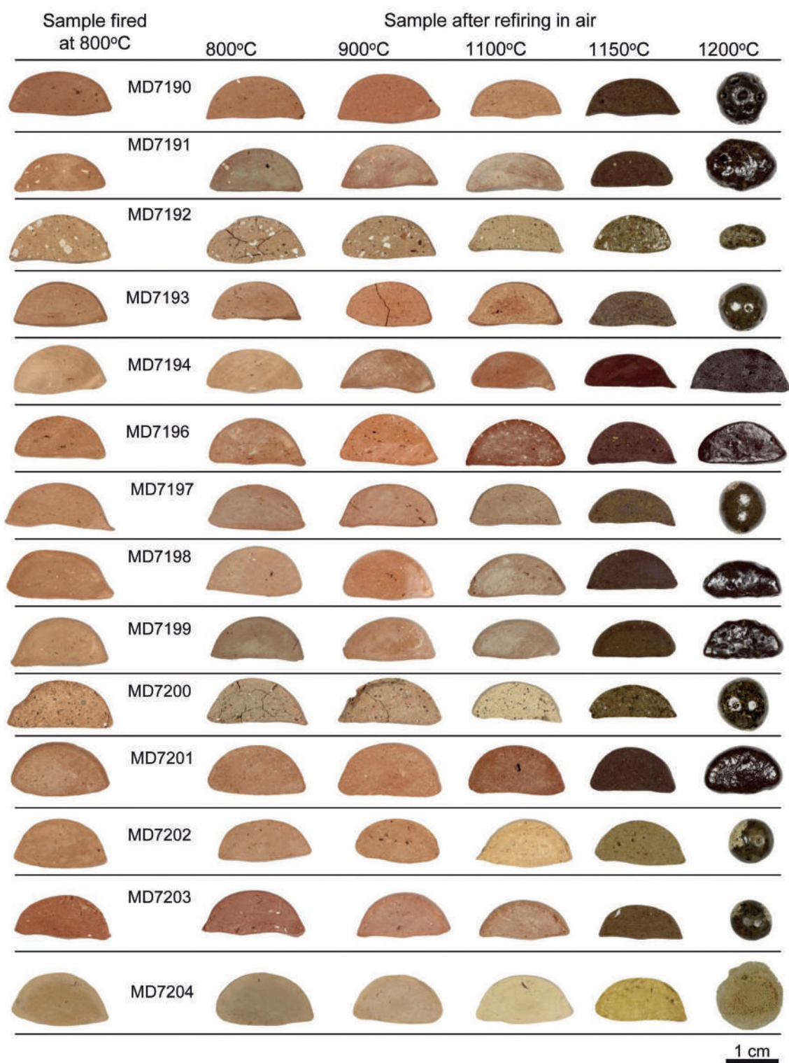
Pl. 14. Test à la ceramics of clay samples MD7190–MD7204, briquettes fired at 800°C (compiled by H. Baranowska and M. Daszkiewicz)
