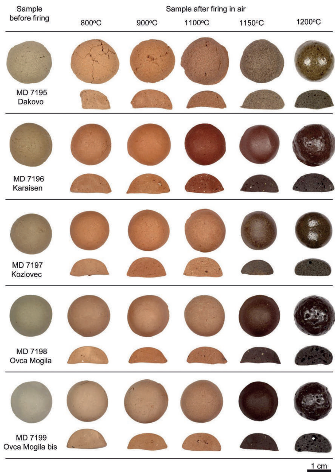
Pl. 12. Firing test, clay samples MD7195–MD7199 (compiled by H. Baranowska and M. Daszkiewicz)
