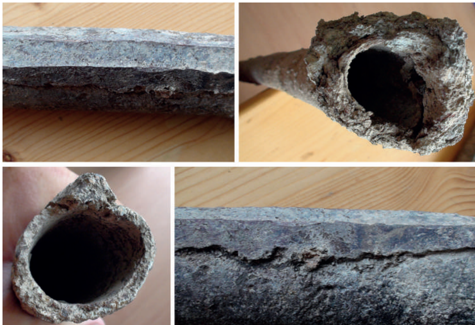
Fig. 4. Close-up of the fistulae: section, folding seam and the ferrule/sleeve (photo by P. Dyczek)
