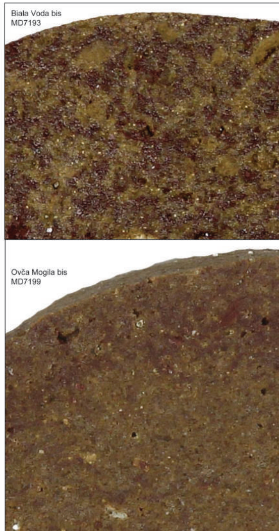
Fig. 12. Briquettes refired at 1150°C of samples made of Bâla Voda Bis and Ovča Mogila Bis clays beforehand fired at 900°C ( à la ceramics test). In both cases a matrix of the “mixed clays of the NC-CC type” is clearly visible; however, this is not a result of the intentional mixing of two types of clay but a feature of the original raw material
