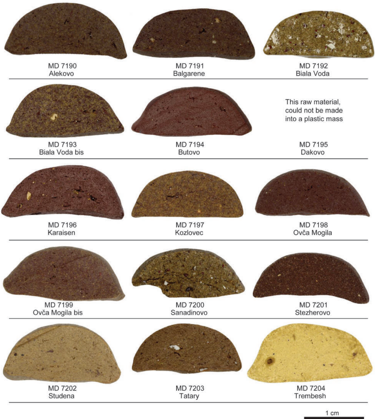
Fig. 10. Cut-sections of briquettes fired at 1200°C (firing test) (compiled by H. Baranowska)
