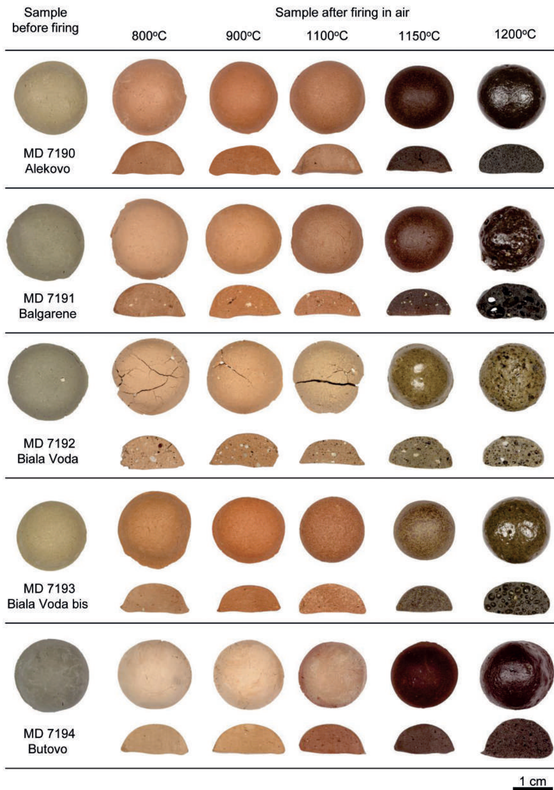
Pl. 11. Firing test, clay samples MD7190–MD7194 (compiled by H. Baranowska and M. Daszkiewicz)
