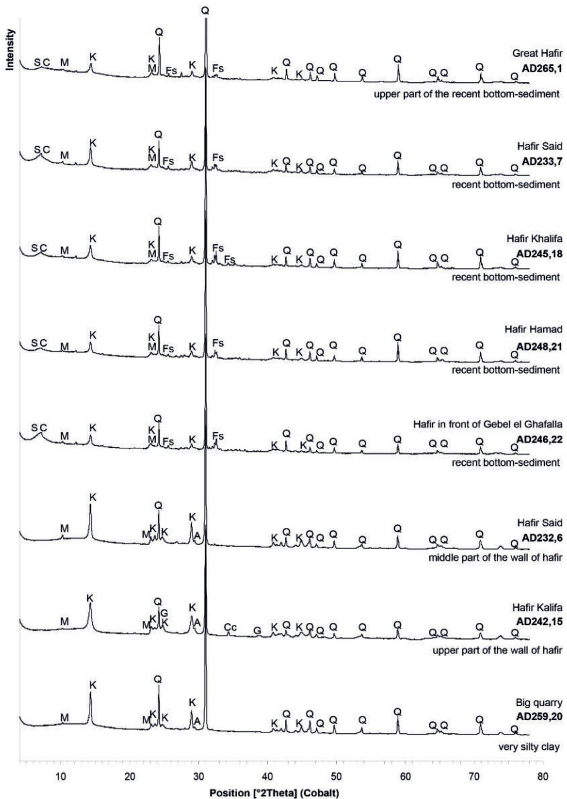
Fig. 19. X-ray powder diffraction analysis of samples taken from various locations:
