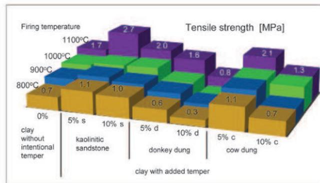
Fig. 34. Tensile strength of briquettes made of wadi clay (AD236) tempered respectively with 5 and 10 weight per cent kaolinitic sandstone, donkey dung or cow dung fired at various temperatures (average values of tensile strength, cv<15%)
