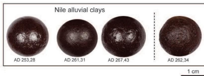
Fig. 17. Specimens of Nile alluvial clays (from left to right: samples taken near Wad Ban Naga, Shendi, El-Geili) and alluvial clay sampled directly from the river bank (AD262,34), fired at 1200°C (macro photos M. Baranowski)
