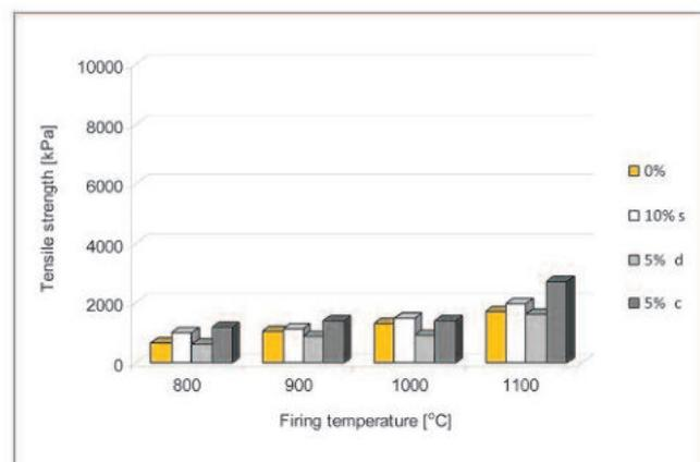
Fig. 33. Tensile strength of briquettes made of wadi clay (AD236) tempered with either kaolinitic sandstone, donkey dung or cow dung fired at various temperatures (average values of tensile strength, cv<15%)
