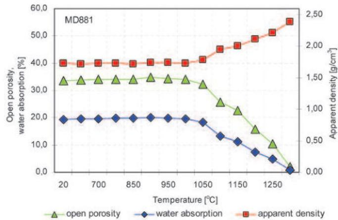
Fig. 36b. Pottery fragment of local Musawwarat wheel-made fine ware. Open porosity, water absorption and apparent density values were estimated at room temperature and after refiring. Original firing temperature  $T_{eq} = ca. 950^{\circ}C$
