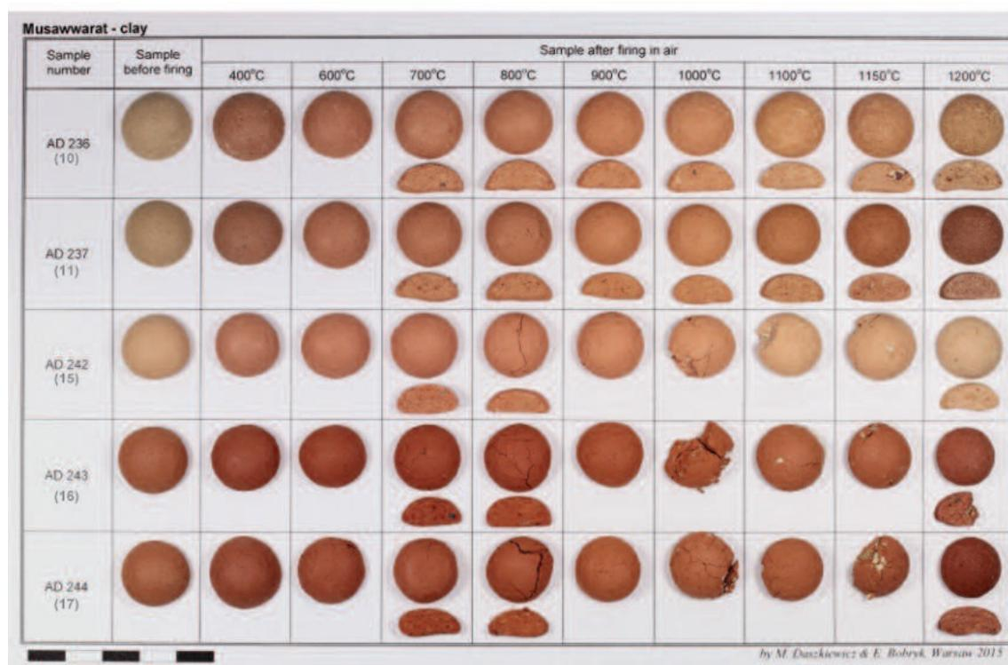
Fig. 15. MGR-chart. Clay specimens before and after firing in air (specimens formed using plastic mass and non-porous porcelain moulds which yielded dome-shaped samples); whole dome-shaped specimens and cut-sections of these specimens (photo M. Baranowski)
