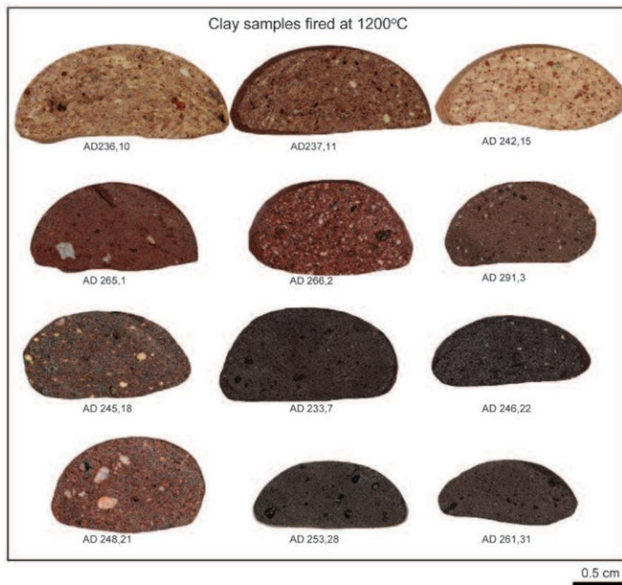
Fig. 18. Cut-sections of specimens of various raw materials fired at 1200°C. Samples of wadi clays AD236,10 and AD237,11 are very similar macroscopically to local Musawwarat fabrics (macro photos M. Baranowski)
