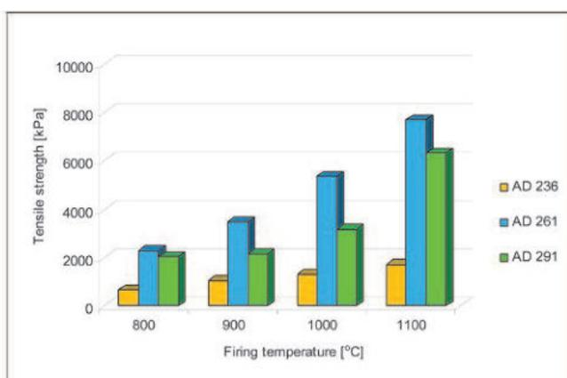
Fig. 31. Tensile strength of briquettes made of wadi clay (AD236), Nile alluvial clay (AD261), clay used by a local potter and clay from the upper layer of the Great Hafir in Musawwarat es-Sufra (AD291) fired at various temperatures (average values of tensile strength, cv<15%)
