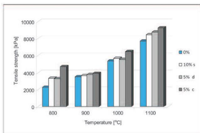
Fig. 32. Tensile strength of briquettes made of Nile alluvial clay (AD261) tempered with either kaolinitic sandstone, donkey dung or cow dung fired at various temperatures (average values of tensile strength, cv<15%)
