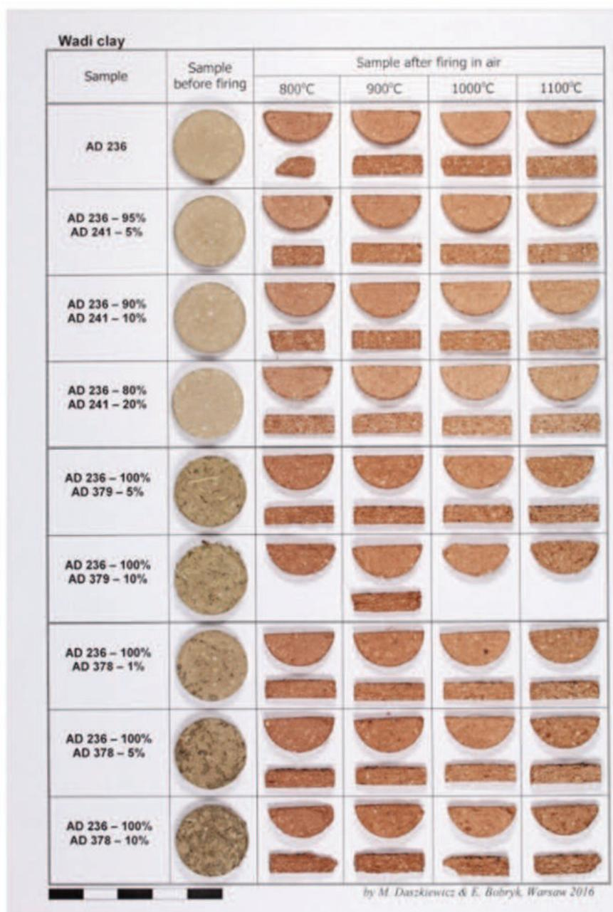
Fig. 29. Briquettes made of wadi clay AD236 tempered with kaolinitic sandstone (AD241), cow dung (AD378) and donkey dung (AD379)
