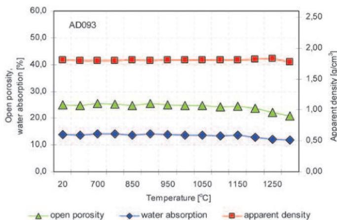
Fig. 36a. Pottery fragment of local Musawwarat wheel-made coarse ware. Open porosity, water absorption and apparent density values were estimated at room temperature and after refiring. Original firing temperature  $T_{eq}$  = ca. 1150°C
