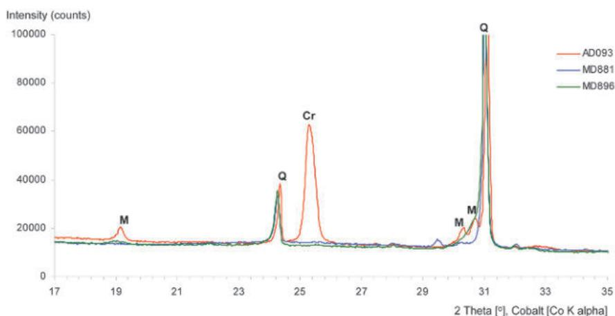
Fig. 35. Diffractograms of X-ray powder diffraction analysis carried out on fragments of local pottery from Musawwarat es-Sufra: M = mullite, Cr = cristobalite, Q = quartz
