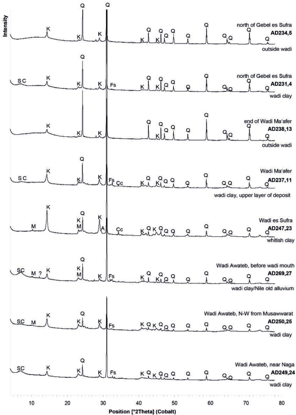
Fig. 20. X-ray powder diffraction analysis of samples taken from various locations:
