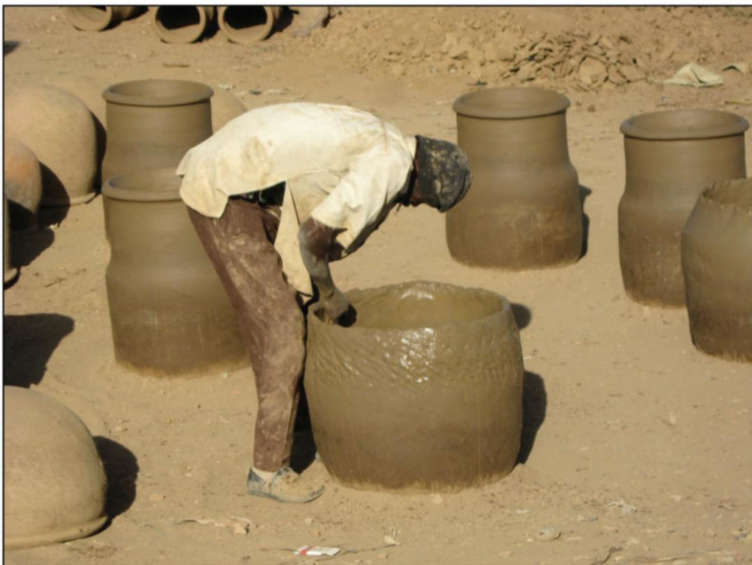
Fig. 4. Orbiting. Potters move around a fixed vessel during both the forming and shaping process. Two pottery workshops at a pottery centre in Wad Medani. Sudan 2008 (photos M. Daszkiewicz)
