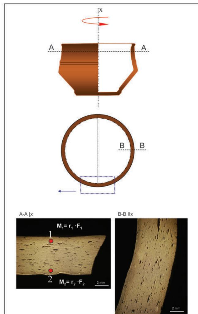
Fig. 8. Pore distribution in a wheel-made vessel. At point 2 pores will be thinner than at point 1 or will disappear due to fact that  $M_2 > M_1$ .  $x$  = axis of vessel; A–A = plane perpendicular to axis of vessel; B–B = plane parallel to axis of vessel;  $M_1$  = moment of force in point 1;  $M_2$  = moment of force in point 2;  $F_1$  and  $F_2$  = pressure exerted by the potter's hand;  $r_1$  and  $r_2$  = radius
