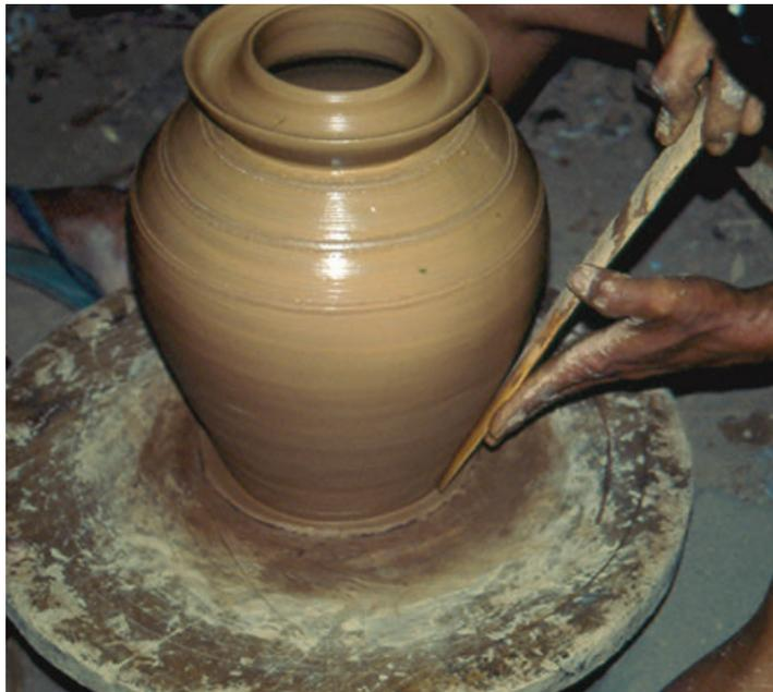
Fig. 6. Wheel-shaped. Coiling: the vessel is built of coils, which are bonded by applying discontinuous pressure, without the help of rotative kinetic energy; thinning and shaping is done with the help of rotative kinetic energy. Hand-operated turntable. Laos 1994 (photos G. Schneider)
