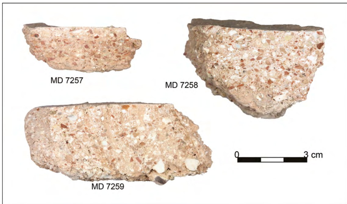
Fig. 7. Samples of lining material taken from a cistern wall (photos M. Baranowski, drawing H. Baranowska).
