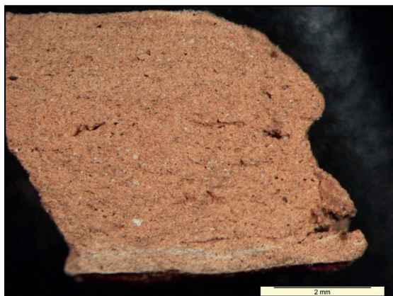
Fig. 2. Fabric A, cross-section of specimen His25/19 under stereoscopic microscope (photo by J. Michniewicz)
