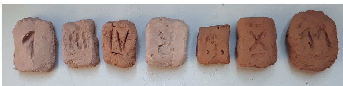
Fig. 11. Clay samples shown in Fig. 10, after firing at 750 °C (photo by J. Michniewicz).
